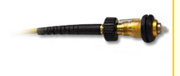
The variable Attenuator Patch Cord provides a compact and simple feature to manually equalize the power of optical signals in fiber optic systems. When mated to a standard connector, the variable attenuator connector causes the optical signal to become attenuated by creating a variable air gap between the connector ferrules. Attenuation is adjusted by means of a selflocking screw mechanism. It ideally fits to the S500 In line power monitor series
