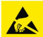
This sign indicates that the respective modules, boards or RF inputs and outputs are susceptible to damage by electro static discharge (ESD), and require proper protection procedures for storage and handling.
